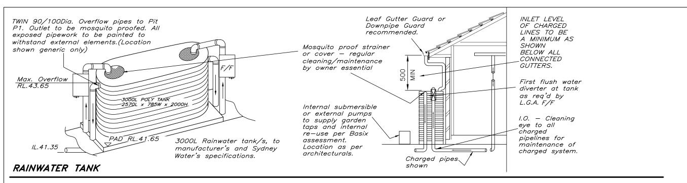
TANK DETAILS SHOWN ARE A SUGGESTED CONFIGURATION ONLY. ANY MODIFICATIONS TO TANK VOLUME OR INLET AND OUTLET LEVELS MUST BE APPROVED BY ENGINEER PRIOR TO COMMENCEMENT OF CONSTRUCTION. TANK SHAPE, & DEVICES SHOWN ARE DIAGRAMMATIC ONLY. MINIMUM OF 450 CLEARANCE (UNLESS L.G.A. REQUIRES LARGER SETBACK) TO SIDE BOUNDARIES MUST BE MAINTAINED. CLIENT IS RESPONSIBLE TO ENSURE COMPLIANCE WITH THIS IN THE INSTALLED STATE. Charged stormwater lines from Roof Areas ONLY to rainwater tank.
